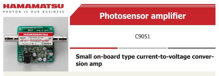
The C9051 is a current-to-voltage conversion amplifier specifically designed for low-light-level measurement using a photodiode (sold separately).
