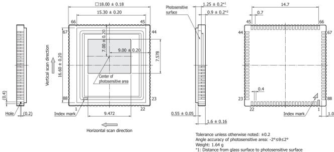
\*1: Distance from glass surface to photosensitive surface
