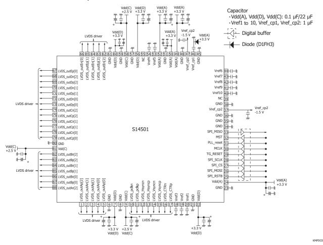
Note: Leave NC pins open; do not connect to GND.
