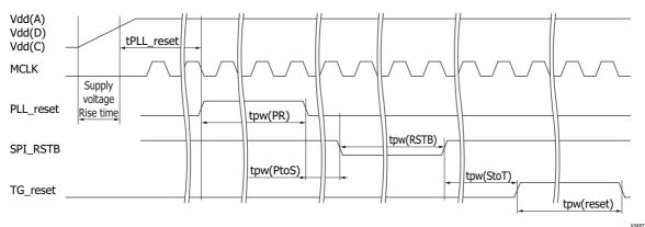
Note: At power-on, input the SPI\_RSTB and Reset signals at the timings shown in the figure above to initialize the timing circuit and SPI circuit after all the supply voltages have risen to the recommended operating conditions [Vdd (A)=Vdd (D)=3.0 V, Vdd (C)=2.4 V].
