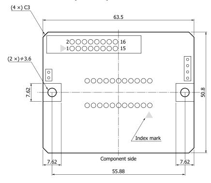
Note: Mount the connector on the component side.
