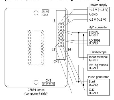
Note: Mount the connector at CN1 on the component side. Install the NMOS linear image sensor into position while aligning pin no. 1 with the index mark (pin no. 1) on the back side of the C7884 series.
