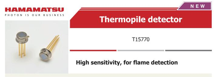
The T15770 is a high-sensitivity thermopile detector suitable for flame detection. Infrared energy generated from flame has spectral characteristics of peak wavelength 4.45  $\mu$ m. The light input window of the T15770 employs the band-pass filter which passes the light of this wavelength.
