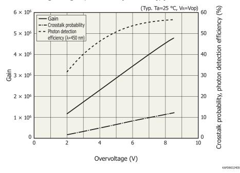
MPPC characteristics vary with the operating voltage. Although increasing the operating voltage improves the photon detection efficiency and time resolution, it also increases the dark count and crosstalk at the same time, so an optimum operating voltage must be selected to match the application.
