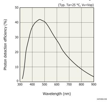
Photon detection efficiency does not include crosstalk and afterpulses.
