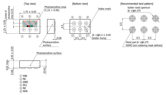
Tolerance unless otherwise noted:  $\pm 0.05$ Solder bump material: Sn (96.5%), Ag (3%), Cu (0.5%)
