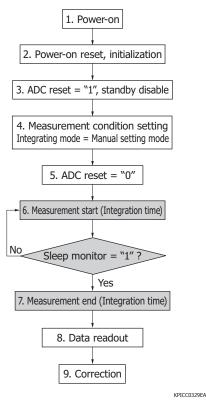
Sensitivity variation can be decreased using the correction coefficient which is calculated from the integration time measurement result.
