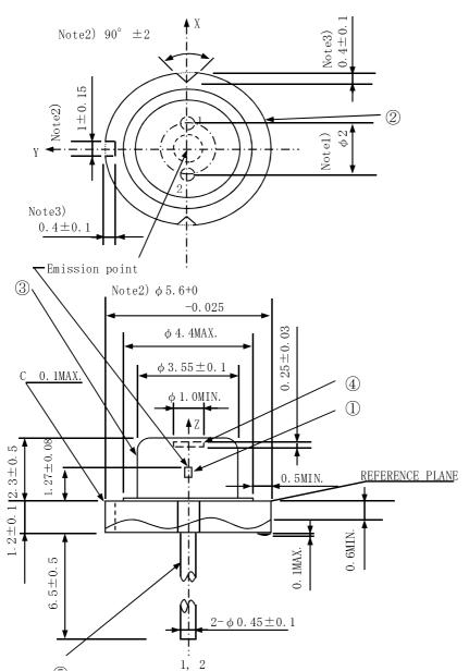
Enlarged drawing around the emission point  $\begin{array}{c} \chi \\ \\ \chi \\ \\ \end{array}$  Emission point  $0 \pm 0.08$   $0 \pm 0.08$
