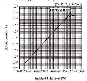
\* This graph does not include the reduction of linearity due to heat.
